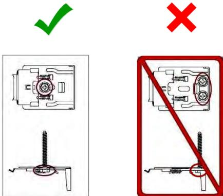
**DO NOT** use hex-head screws for holes on the back of the bracket for inside mount. It will prevent your shade from clicking in place. These holes can be operated with 2 flat-head screws (Flat-head screws are not included in the package).
