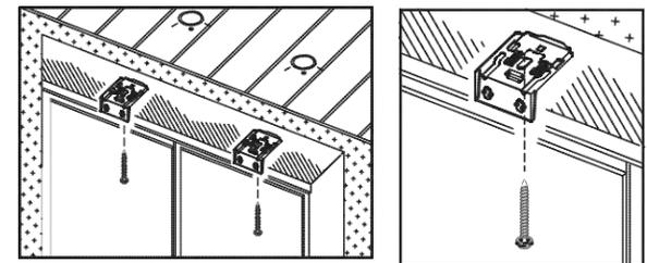
Make sure both brackets are aligned. "L" shape opening should be facing down, with longer side against top of the window opening.
